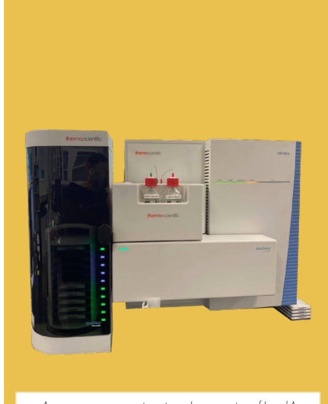
A paper spray mass spectrometer — Image courtesy of Jarred Aasen
